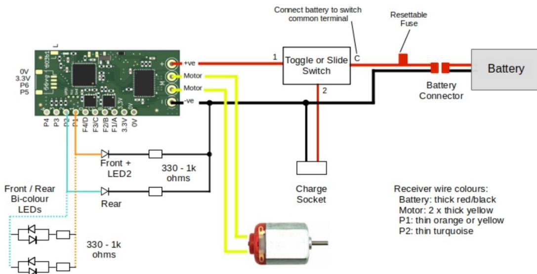
LEDs on P pads should be connected between the pad and battery negative (0V) with a series resistor appropriate to the required brightness.
