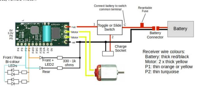
LEDs on P pads should be connected between the pad and battery negative (0V) with a series resistor appropriate to the required brightness.
