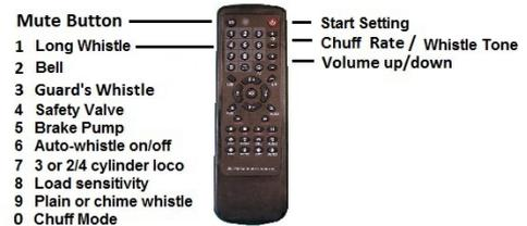
Adjustments to the sounds can then be made without taking the loco apart to access the sound module.
