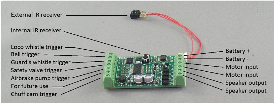
The MyLocoSound module generates synthesised sound which is adjustable to reproduce the sounds of most steam locos and railmotors. The terminal connections on the right are necessary for the sound module to generate a chuff which varies with the loco speed and load. The terminal connections on the left trigger the various sounds where the locomotive controller has the appropriate outputs available
