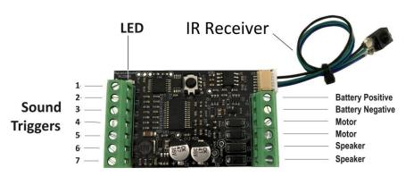
various sounds where the vehicle controller has the appropriate outputs available. The trigger terminals are labelled F1 to F7 and are referred to by these labels in these instructions. For example, "Triggering F1" means to close a contact between the F1 terminal and the Battery negative terminal.
