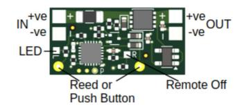
MSW11a is available as: a bare board with reed switch mounted; or without reed switch mounted (e.g. for use with a push button); and with optional input, output and charge connector wires.
