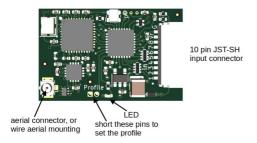
The JST-SH 6p, pin 3 can power an external LED which mirrors the on-board LED. The external LED needs a series resistor suitable for 3.3V - see one of the wiring diagrams below for an example LED connection. The on-board LED is turned off after 30 seconds.
